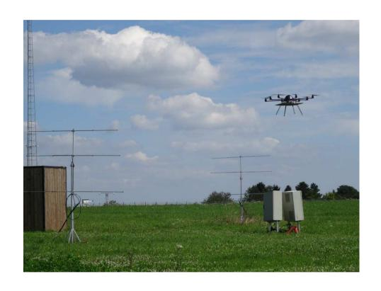
Using the BRAMS calibrator as Tx (payload) to test the direction retrieval algorithm
