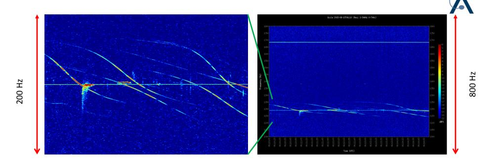
The frequency of the BRAMS calibrator is very stable ( $\sim$ few Hz) which is much better than the one of the LO of the receiver (that can drift up to 200 Hz depending on temperature). Frequency drifts of LO will affect beacon and calibrator frequencies in the same way such that the frequency range between them  $\sim$  500 Hz.
