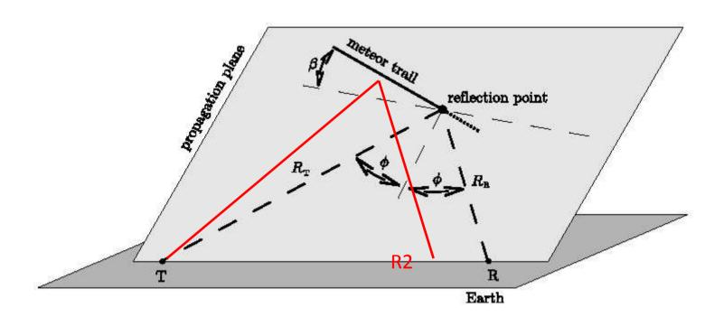
Ionisation in several points → estimate of mass of meteoroid using ablation model (complex inverse problem, collaboration with VKI)
