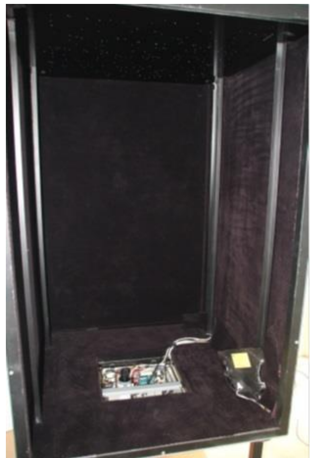
Figure 3 – Picture of the unit of calibration. The front pannel was detached during the picture. The unit concept is that the entire experiment simulates an ideally dark night.
