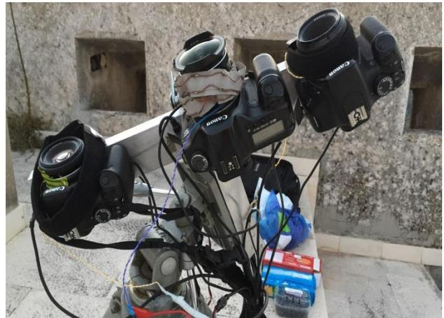
*Figure 1* – Setup of the CHIPOIAtA system: 2x Canon EOS 550D with Nikkor 50mm F/2 lens, aligned such that they form one long FoV. In between camera and lens the optical choppers are mounted (not visible). In the center a third (All-sky) camera is visible (also with optical chopper), but not being part of CHIPOIAtA.
