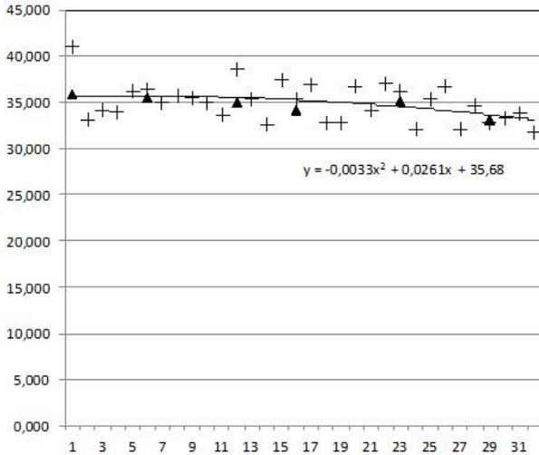
Figure 4 – Velocity profile for the measured data points. Vertical axis velocity in km/s; horizontal axis arbitrary break number. Crosses refer to single data points, solid triangles to a 6-pt average. The solid line represents a polynomial fit. There is evidence for deceleration.
