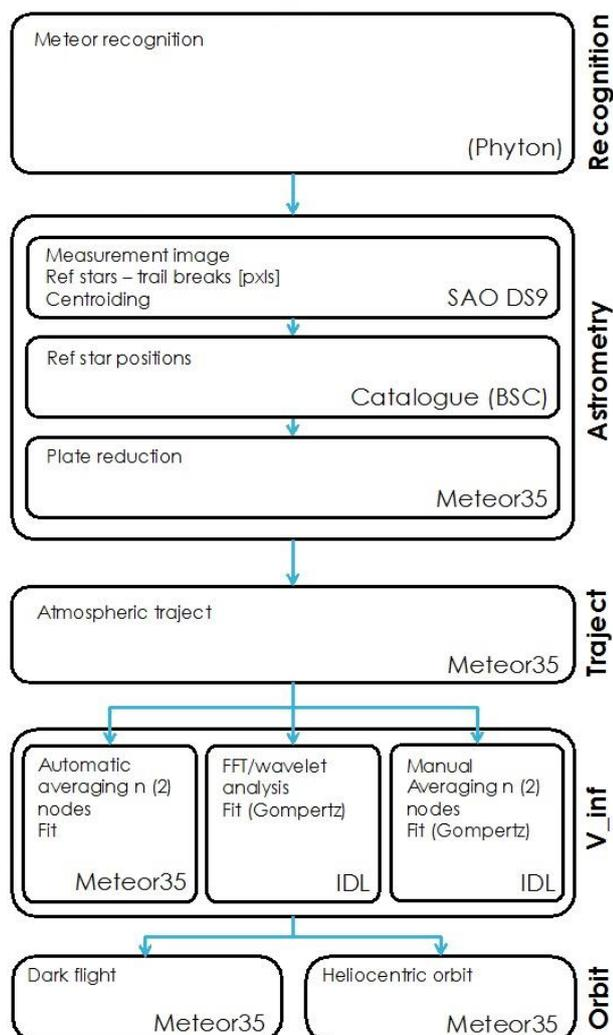
Figure 5 – Schematic pipeline for the data reduction.
