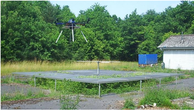
Figure 2 – UAV flying around the antenna beacon at Dourbes.
