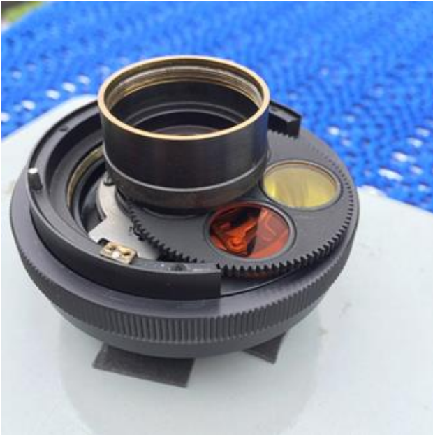
Figure 8 – The ‘heart’ of the fisheye lens with front and rear lens groups taken away and internal filterwheel now clearly visible, ready for replacement by the electronic chopper.
