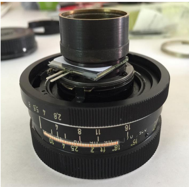
Figure 9 – Side view with the LC-TEC optical shutter instead of the filterwheel in place now.
