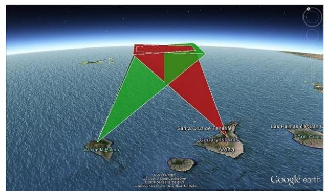
*Figure 1* – CILBO double station camera setup including the fields of view of both cameras and the overlapping volume in which simultaneous meteor detections are feasible. Camera ICC9 is located on La Palma (left island) and camera ICC7 on Tenerife (right island). The setup was generated using Google Earth. (Drolshagen et al., 2014).
