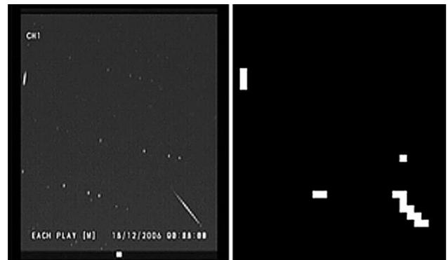
Figure 6 – Top-left: max pixel for test data of two meteors. Top-right: thresholded and subsampled image. Bottom: 3D line finding algorithm results.
