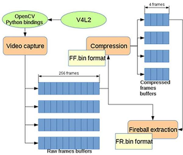
Figure 3 – Processing pipeline.
