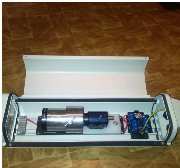
Figure 2 – Station Kroměříž, NFC system in its housing.
