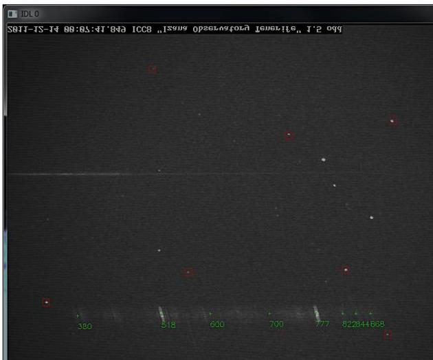
*Figure 4* – Illustration of the spectral data processing pipeline. The meteor position is read from the \*.inf file produced by MetRec via camera ICC7 and tick marks are generated for different selected wavelengths.
