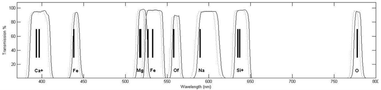
Figure 2 – Composite of filter scans for both normal incidence (solid) and 12 degrees off-axis incidence (dotted) with targeted meteor emission lines (bold vertical lines).
