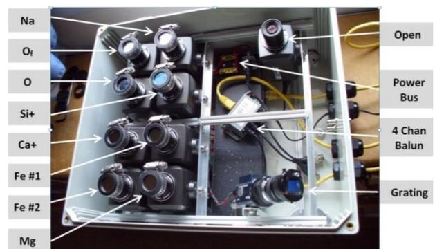
Figure 3 – Completed system of filter bank and grating.
