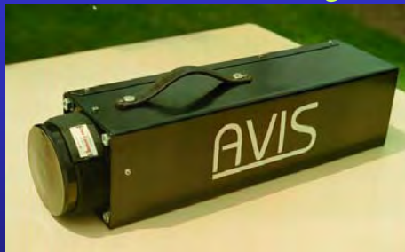
Image-intensified camera Fov 60°, lm +6 mag
