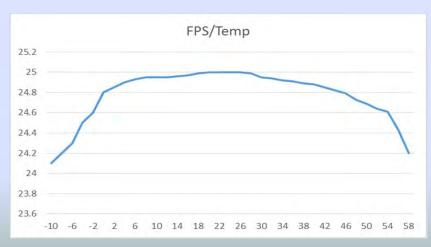
For WATEC 902U cameras, the range temperature is even narrower, thus functioning relatively correct up until 51 C, with a shift that adds up to 1.42 FPS. The temperature variations of the camera also affect the performance of the CCD sensor, so that the intern noise variation between winter and summer can gain significant importance in determining the sensibility of the whole video system.
