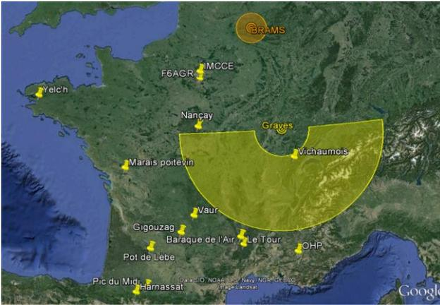
Figure 2 – Locations of BRAMS and GRAVES transmitters. The yellow pins show the various receiving places which have already successfully been tested with low gain receiving antennae.
