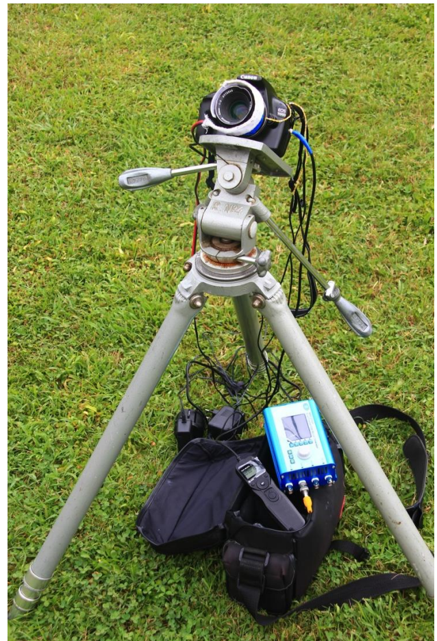
Figure 1 – Setup of the high-resolution camera: Canon EOS 1100D with Nikkor 50mm F/2 lens and in between (not visible, LC-TEC X-FOS(G2) optical shutter. The function generator for shutter control is visible below the tripod (in blue), as well as an exposure controller.
