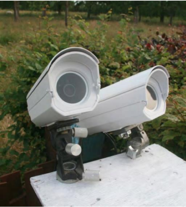
Figure 1 – Station Wildert. The cameras typically are mounted in weatherproof video surveillance casings, being cheap and making realization of a new station an easy exercise.
