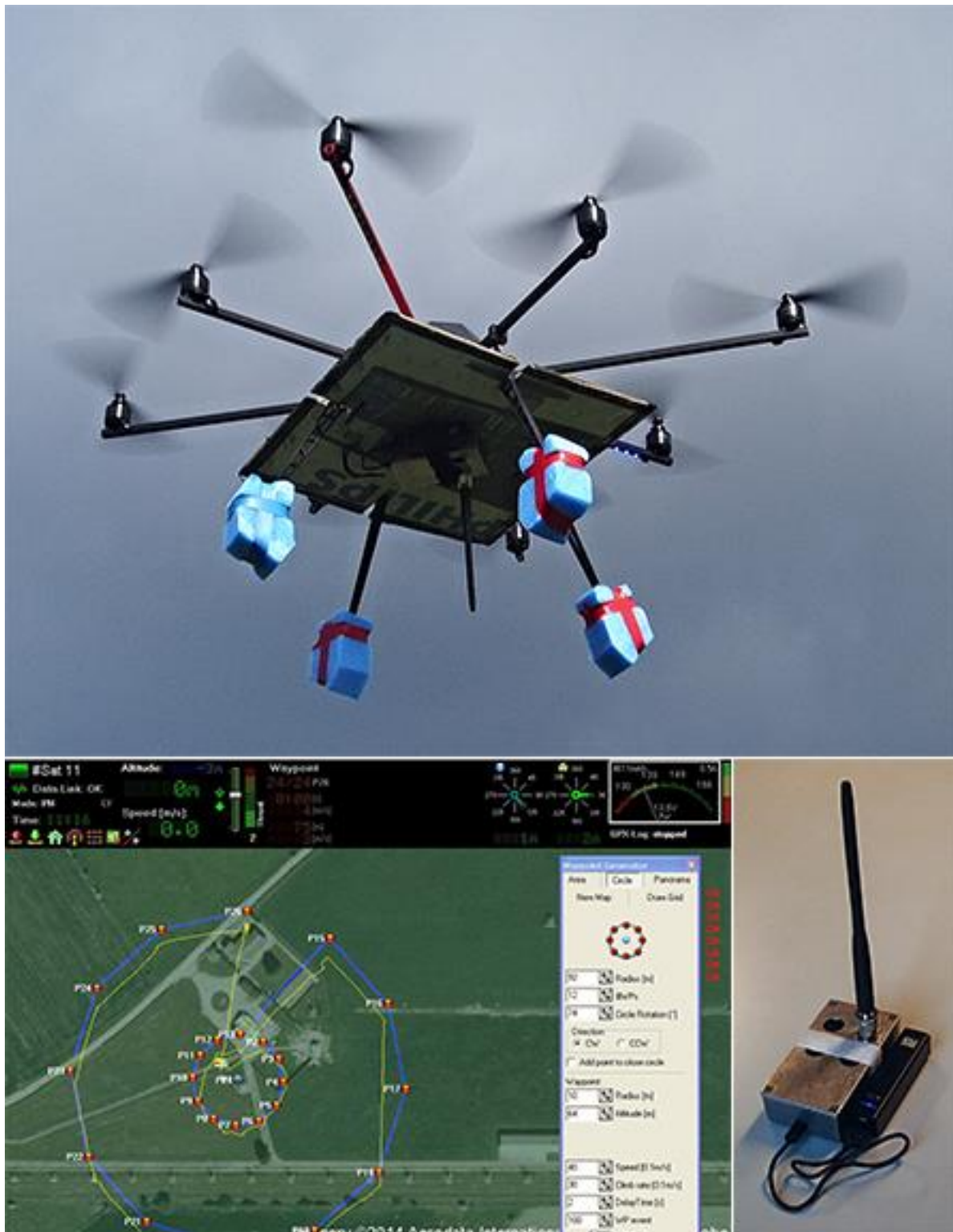
Figure 6 – Measurement system (Top: UAV OktoXL in flight equipped with RF signal generator, battery bank, transmitting antenna and isolating metallic mesh; bottom-left: Screenshot of the control software with the flight plan and the tracking of the actual flight; bottom-right: RF signal generator).
