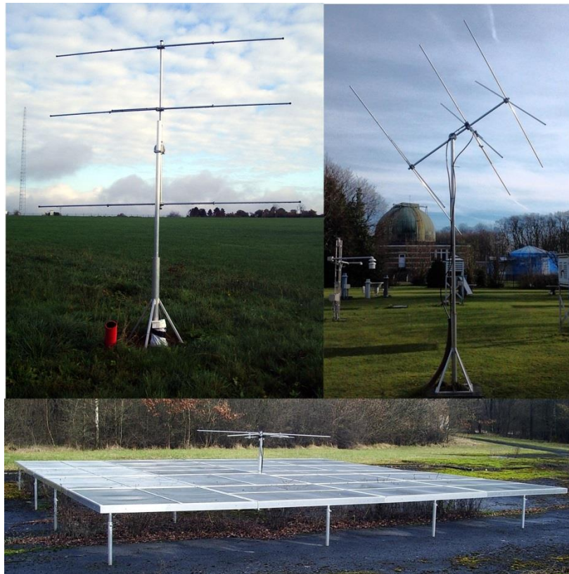
Figure 2 – Images of BRAMS antenna systems directly managed by BISA (Top left: Yagi at Humain Radio Astronomy Station. Top right: Crossed Yagi at BISA facilities, Uccle. Bottom: Turnstile at Dourbes Geophysical Centre).
