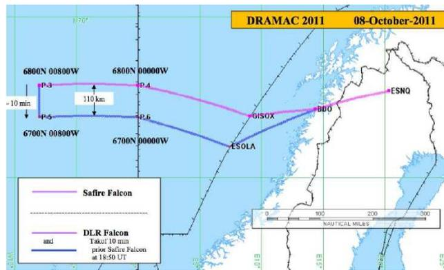
Figure 2 – Flight plan covering the second peak.
