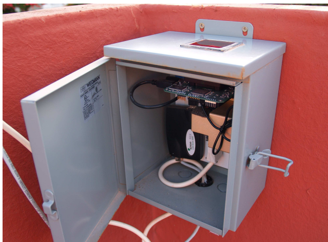
Figure 1 – The all-sky camera. (SMA)
