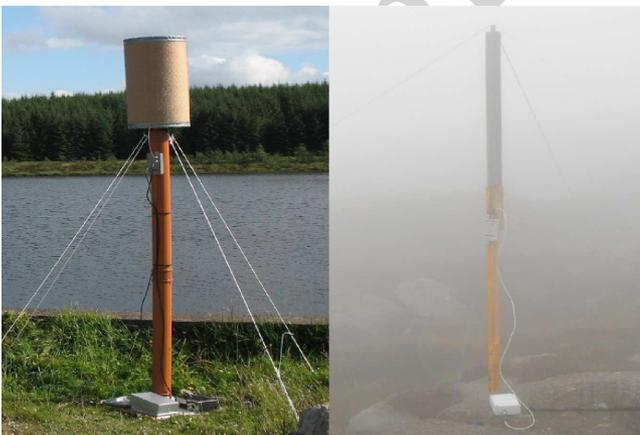
Figure 2 – ELF/VLF antennas used at Armagh Observatory.
