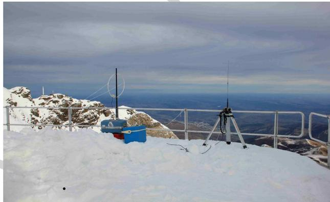
Figure 4 – VLF magnetic loop and VHF vertical whip antenna installed at Pic du Midi Observatory for the Geminids 2011 campaign.
