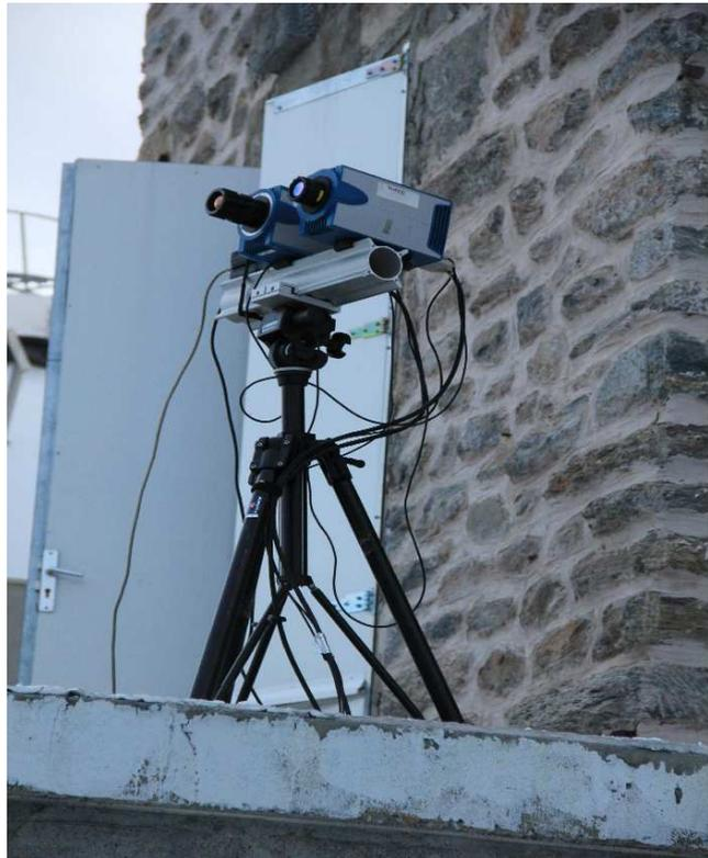
Figure 3 – ONERA 3 and 11  $\mu\text{m}$  cameras under test at Pic du Midi Observatory during the Geminids 2011 campaign.
