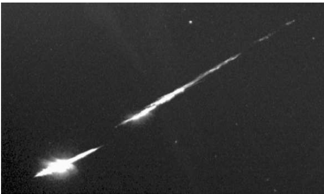
Figure 1 – Composite image of the SPMN061211 ORN fireball recorded together with its emission spectrum from El Arenosillo meteor observing station on December 6, 2001, at 20^{\text{h}}32^{\text{m}}59^{\text{s}}.4 \pm 0^{\text{s}}.1 UT. Note that the zero-order image is close to the bottom-right border.
