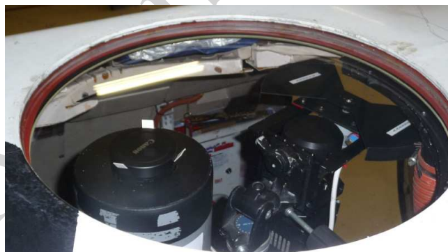
Figure 4 – Upper window of the DLR Falcon plane. The AMOS camera is on the left.
