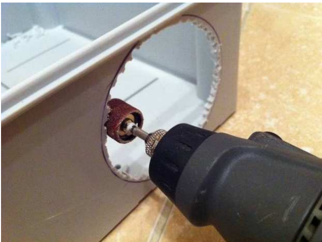
Figure 5 – Opening cut out for the UV filter.
