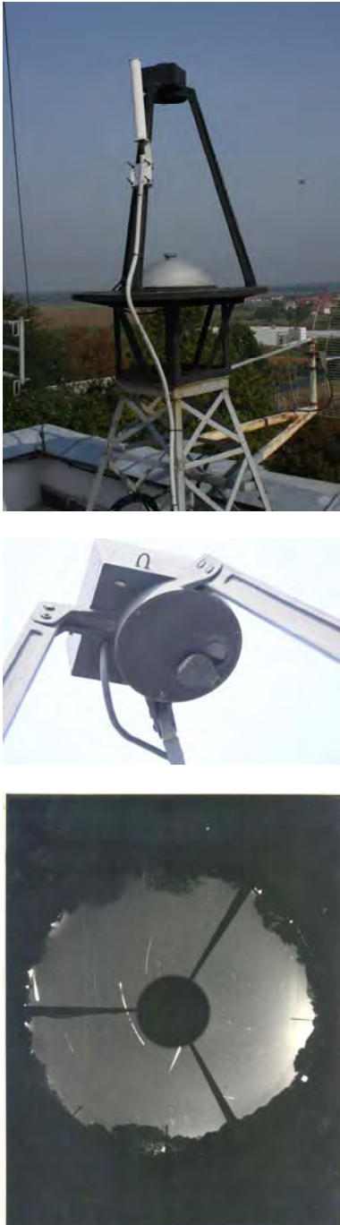
Figure 3 - All-sky camera at the tower of the Slovak Hydrometeorological Institute, Hurbanovo (top and middle panels) and Image recorded by the photographic all-sky camera from the archive of the SCO (bottom panel).
