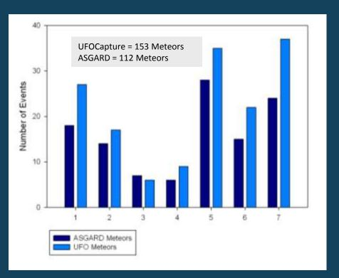
Lowered Threshold (from 75 to 50) and removed a rejection filter that flagged a bunch of single frame triggers (meant for blinking planes).
