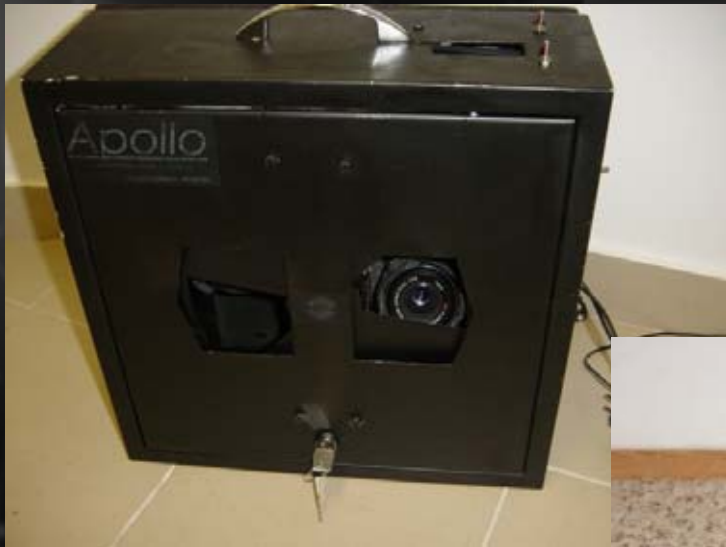
APOLLO, PHAETHON and TOUTATIS – rotating shutters used during this campaign
