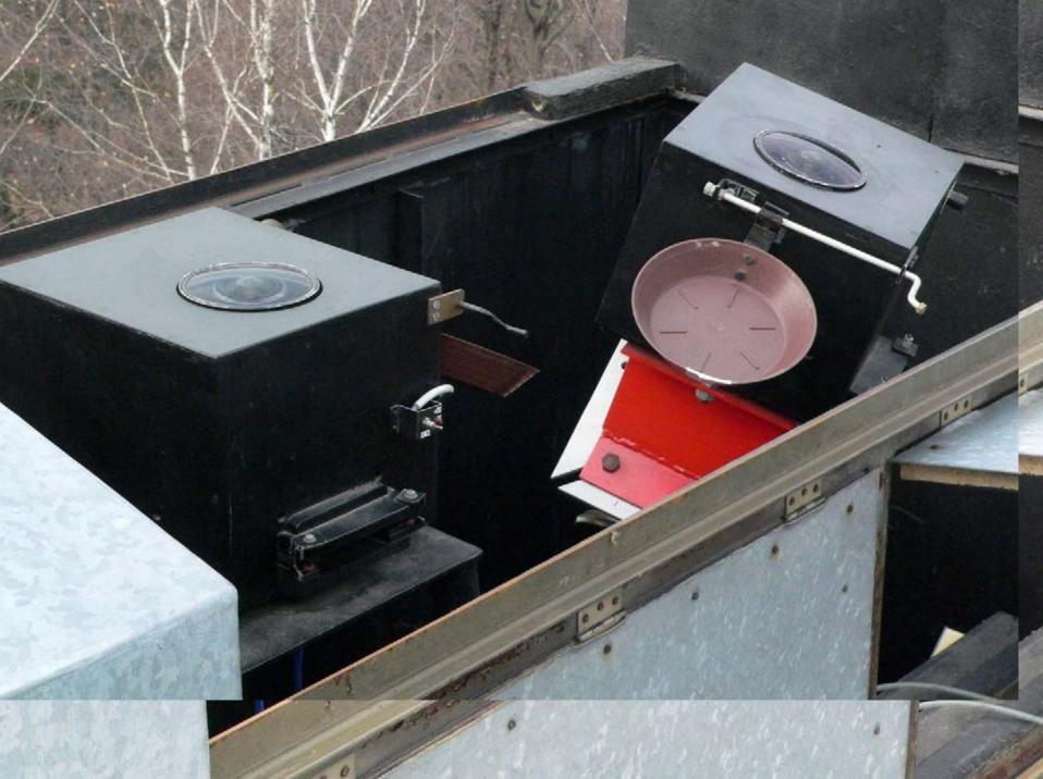
Forward scatter radio system Bologna-Modra-Lecce for meteor observation frequency 42.7 MHz (CNR, Italy)
