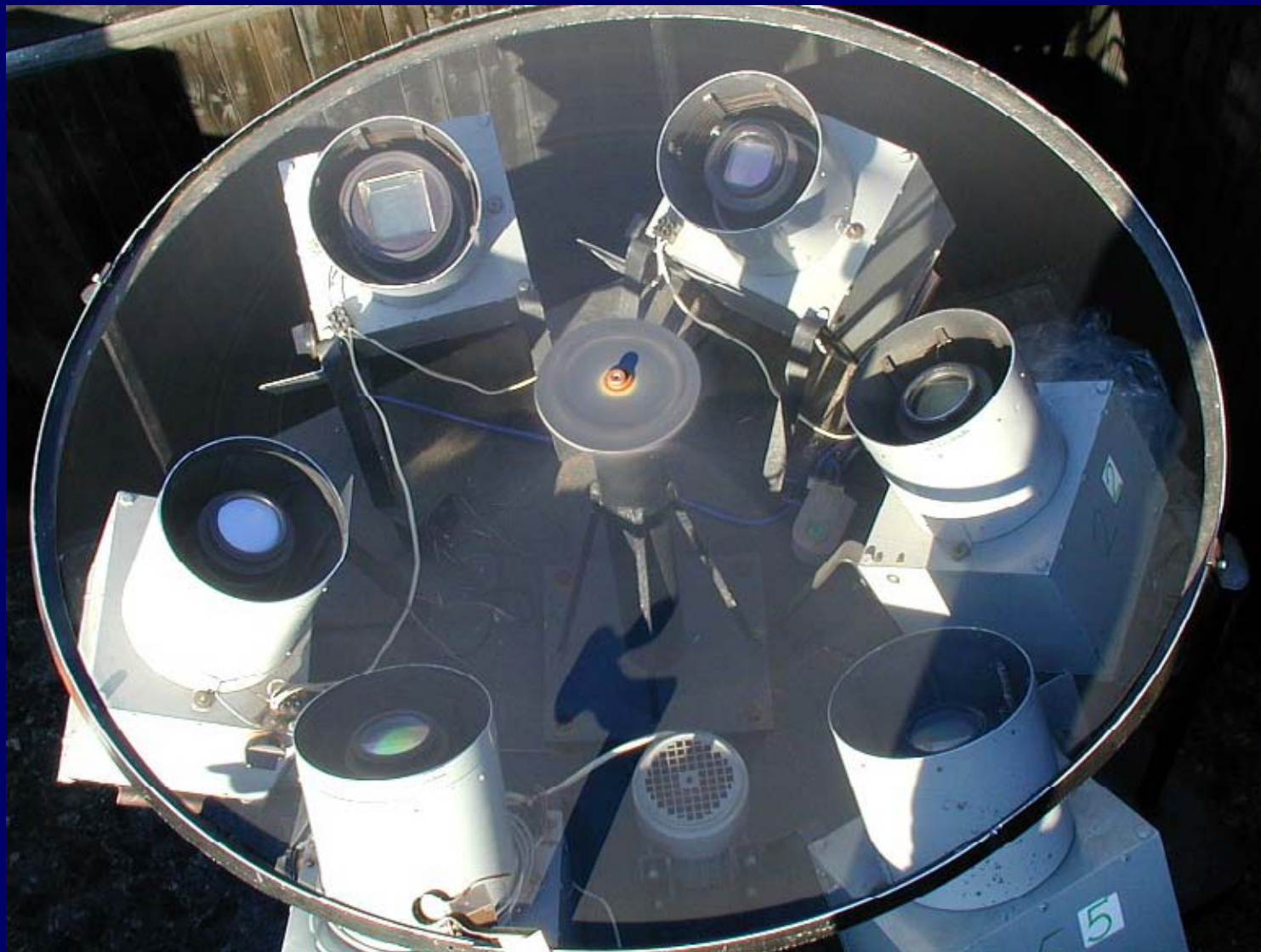
Battery of six photographic grating cameras with rotating shutter in Ondřejov
