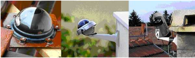
Figure 3 – The “evolution” of CMN camera cases, starting with the basic (left) to the currently used (right).
