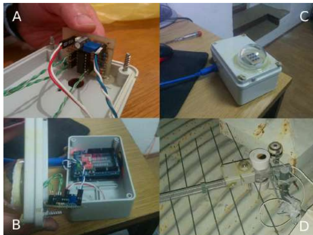
Figure 1 – Meteor radiometer hardware setup. A) Amplifier board with a 4 channel LMC6464 amplifier. Three triples of BPW34 photodiodes are connected to individual channels, their signals are amplified, summed, and amplified again through the fourth remaining channel. B) Amplifier board is packed in a box with an Arduino-based DAQ. C) Nine photodiodes are protected by an acrylic dome. D) The radiometer is mounted next to an SQM meter and an all-sky camera.
