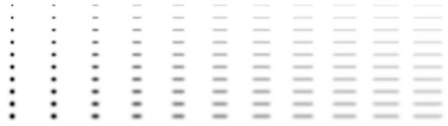
Figure 7 – Simulated star trails for different variances (from 1 in the first to 10 in the last row) and velocities (from 0 in the first to 50 in the last column).
