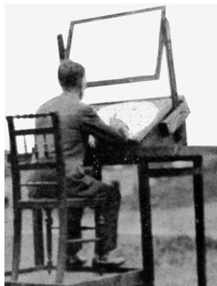
Figure 1 – Plotting through the mirror according to J. Svoboda. (From Říše hvězd X (1929), p.142.)
