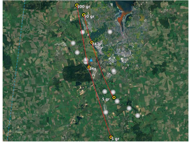
Figure 6 – Expected dropping locations for a 24 gram fragment created at 45 km height, in the case we vary all unknown input parameters within a certain range (Table 3), and use estimates for the parameters which we would not know if no meteorite was found yet (i.e. density 2000–3000 kg/m 3 ). The yellow dots and red lines are overlotted from Figure 5.
