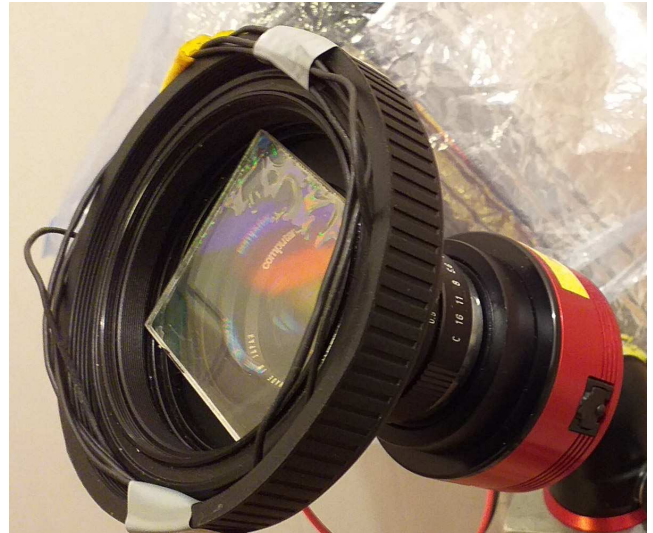
Figure 1 – General arrangement of the grating mounting.
