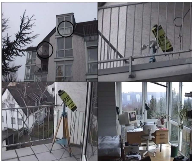
Figure 1 – The start of the IMO Video Meteor Network at my Aachen flat in March 1999 (top left). The camera AVIS was installed on the balcony (top right, bottom left) and fed the video signal live into the analysis computer (bottom right).
