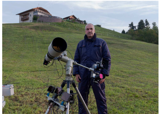
Figure 7 – Setup for project 3CAMPI – CF (3-Camera Measurement of the Population Index with Concentric Fields for the Perseids 2021). Camera 1 was equipped with a Sony GM 1.4/24 mm, camera 2 with a Zeiss Planar 1.4/85 mm and camera 3 with a Canon 2.8/400 mm tele lens.
