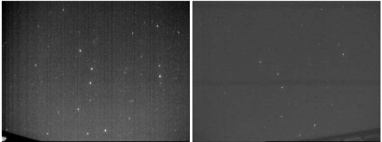
Figure 3 – Reference image of the Watec 910HX-RC (left) and the Mintron 12V6-EX cameras (right), averaged over 64 video frames.
