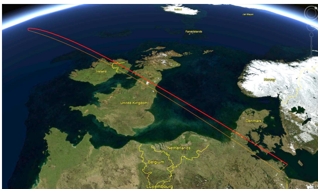
Figure 7 – An illustration showing the full atmospheric flight path (red on the electronic colour version) for the fireball, and its projected surface track (orange – including a linking line to indicate its start elevation), against the spheroidal Earth. Diagram created using Google Earth.
