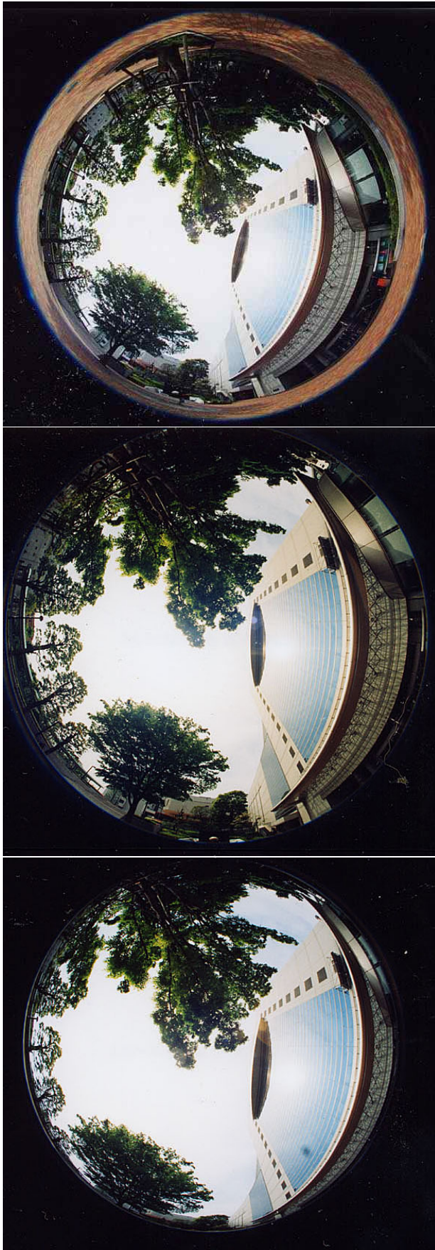
Figure 5 – Images of made with 3 different fisheye lenses: (a) Equidistant 6 mm with 220° FoV, tiles on the street are visible. (b) Equidistant 8 mm with 180° FoV, tiles are not visible anymore, the edge of the image equals horizon. (c) 10 mm orthographic lens, the image compresses strongly towards the horizon, the scale decreases to zero at the horizon.
