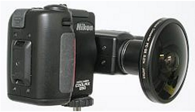
Figure 6 – Nikon Coolpix 4500 with FC-E8 fisheye converter.
